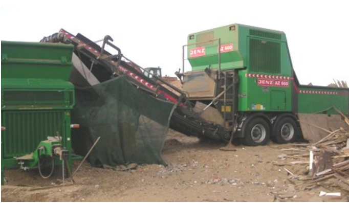
▲ A high volume wood chipping machine.
